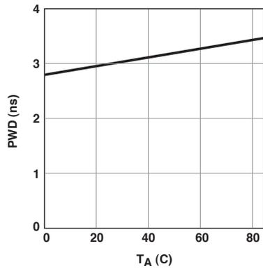
Figure 4. Typical pulse width distortion vs. temperature
