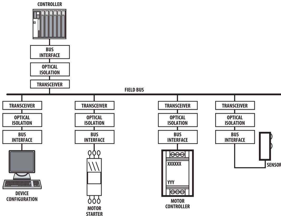
Figure 17. Typical field bus communication physical model
