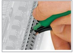
Inserting a conductor via 3.5 mm screwdriver.
