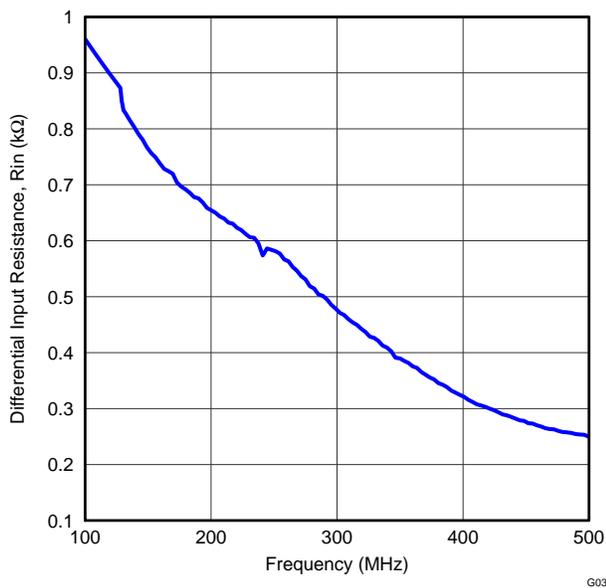
Figure 44. ADC Analog Input Resistance ( $R_{IN}$ ) vs Frequency
