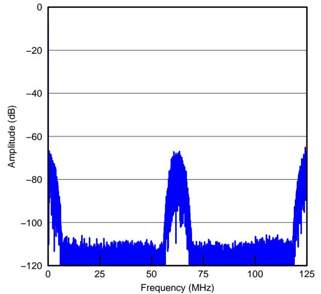
**Figure 60. 45-MHz SNRBoost<sup>3G+</sup> Filter Bandwidth Centered on  $f_S / 8$  and  $3 f_S / 8$**
