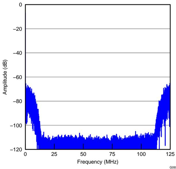
**Figure 59. 90-MHz SNRBoost<sup>3G+</sup> Filter Bandwidth Centered on  $f_S / 4$**
