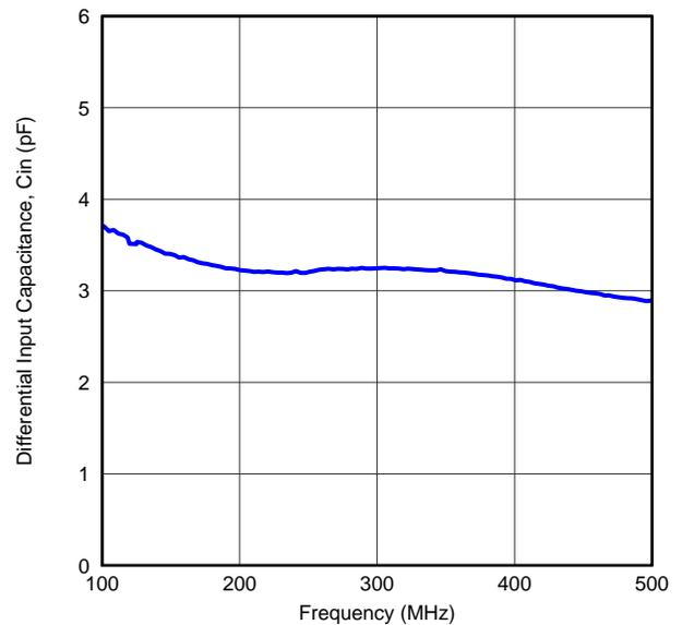
Figure 45. ADC Analog Input Capacitance ( $C_{IN}$ ) vs Frequency
