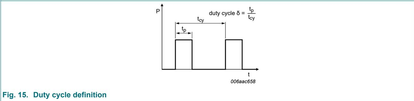
Fig. 15. Duty cycle definition
