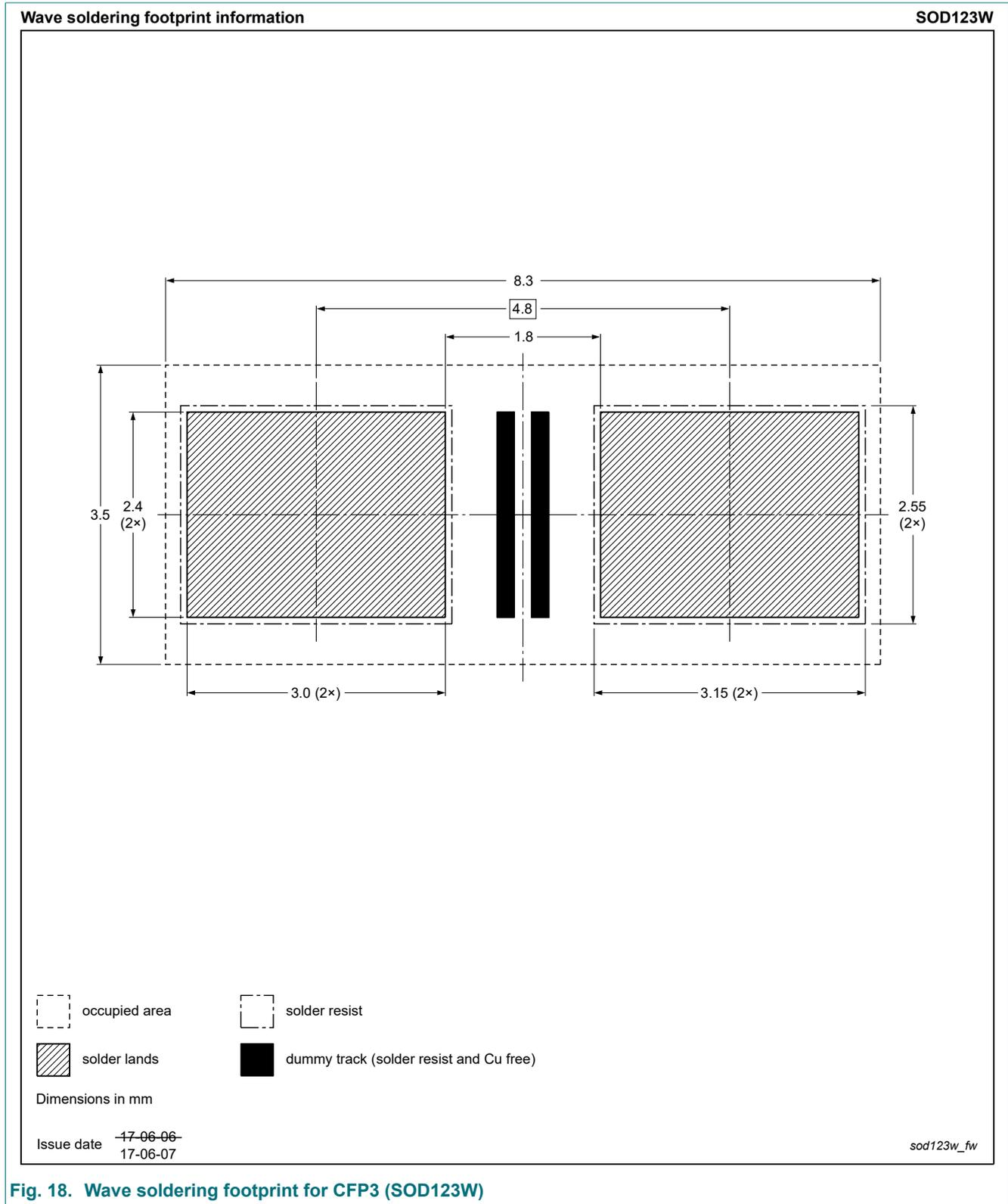
**Fig. 18. Wave soldering footprint for CFP3 (SOD123W)**
