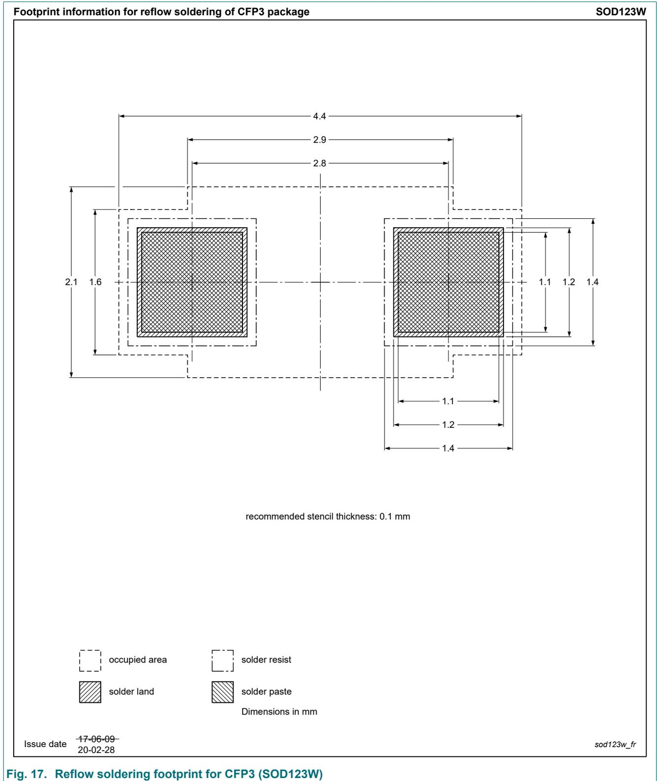
Fig. 17. Reflow soldering footprint for CFP3 (SOD123W)
