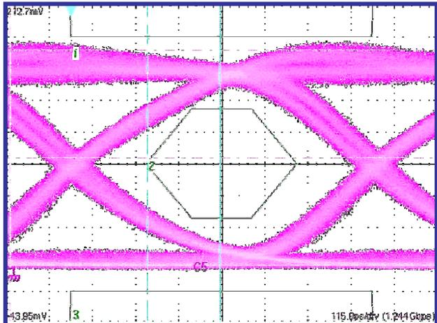
Figure 10. Filtered 1244Mbps Output Without Compensation Network
