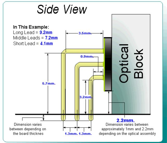
Figure 5. Lead Length Diagram (HFRD 10.2)
