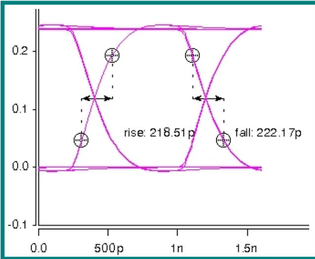
Figure 8. Simulation Result with No Compensation Network
