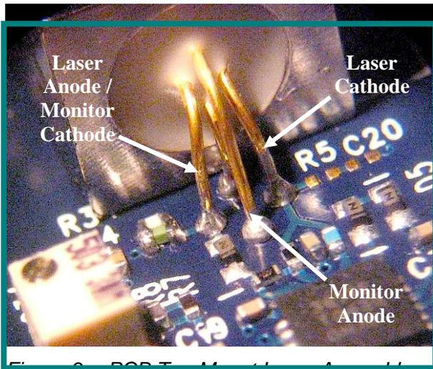
Figure 3. PCB Top Mount Laser Assembly (Laser Connection Detail)
