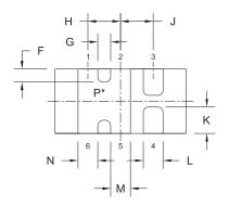
BOTTOM VIEW R2 \* Exposed pad P connects pins 1, 2, 5, and 6.
