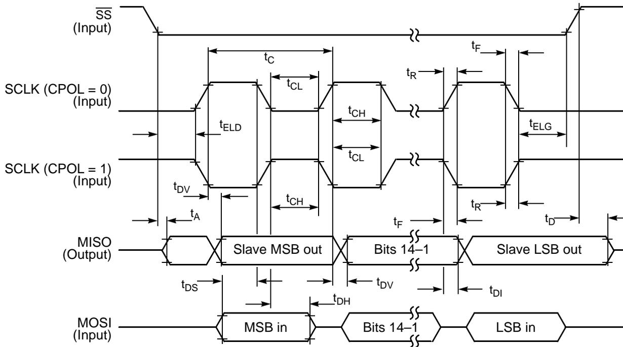
**Figure 3-22 SPI Slave Timing (CPHA = 1)**
