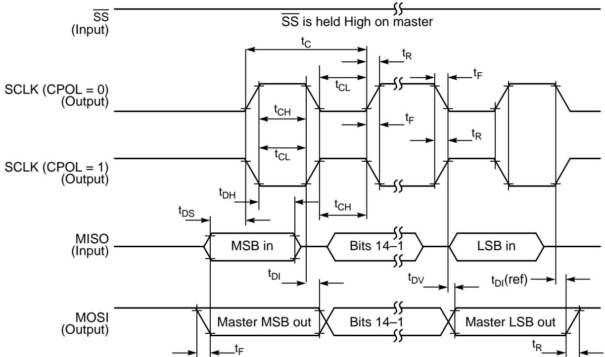
**Figure 3-19 SPI Master Timing (CPHA = 0)**
