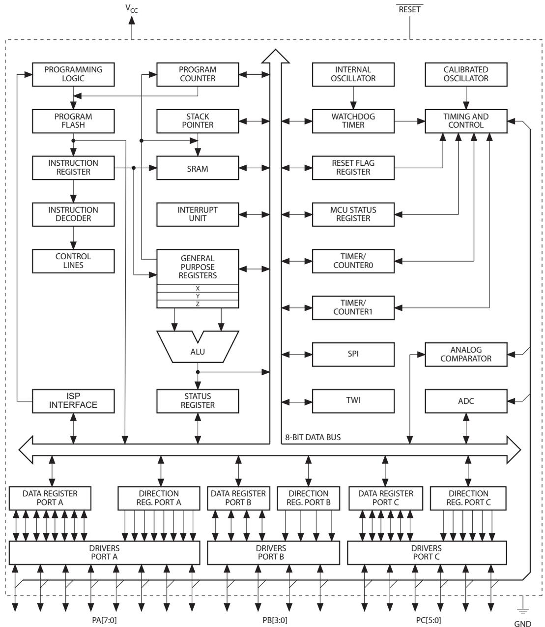
accessed in one single instruction executed in one clock cycle. The resulting architecture is compact and code efficient while achieving throughputs up to ten times faster than conventional CISC microcontrollers.
