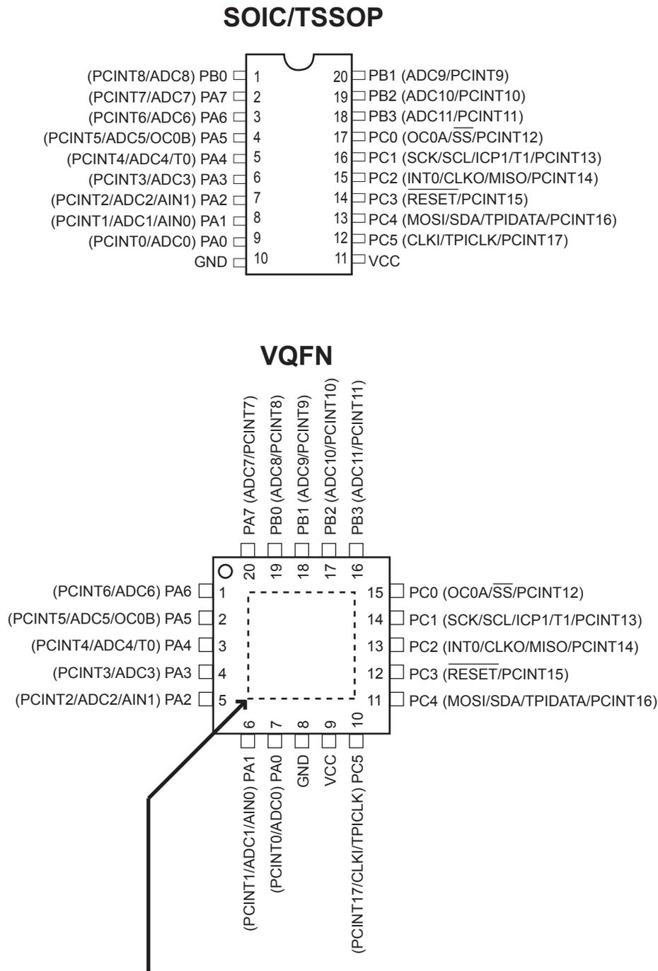
NOTE: Bottom pad should be soldered to ground.
