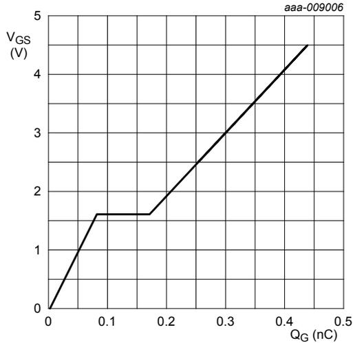
$I_D = 0.6 \text{ A}; V_{DS} = 10 \text{ V}; T_{amb} = 25 \text{ }^\circ\text{C}$
