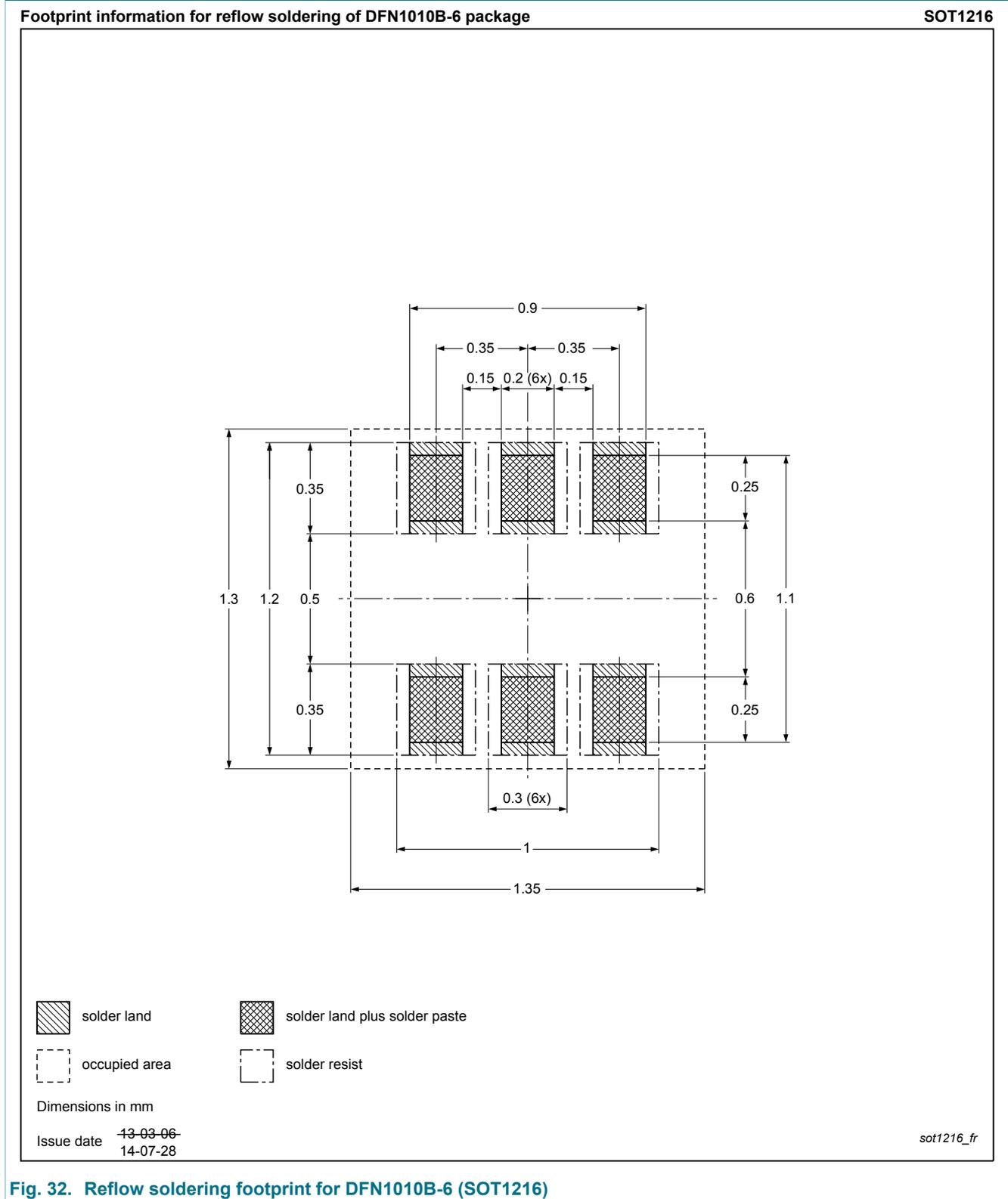
Fig. 32. Reflow soldering footprint for DFN1010B-6 (SOT1216)
