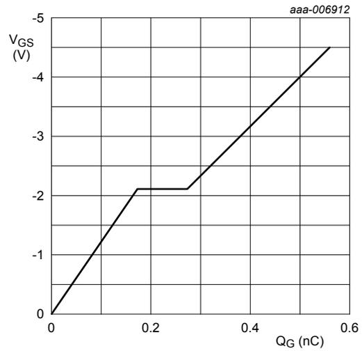
I<sub>D</sub> = -0.45 A; V<sub>DS</sub> = -10 V; T<sub>amb</sub> = 25 °C
