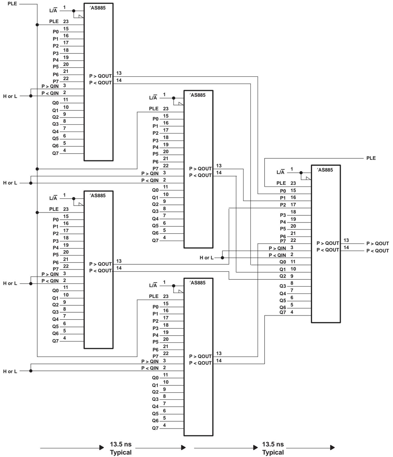
Figure 1. 32-Bit to 72 (n)-Bit Magnitude Comparator
