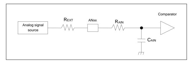
(Equation 1)  $t_S \ge (R_{AIN} + R_{EXT}) \times C_{AIN} \times 9$
