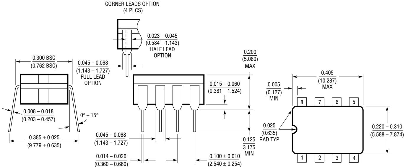
NOTE: LEAD DIMENSIONS APPLY TO SOLDER DIP/PLATE OR TIN PLATE LEADS.
