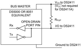
$R_{\text{PUP}}$  must be between 0.3 k $\Omega$  and 2.2 k $\Omega.$  The optimal value depends on the 1-Wire communication speed and the bus load characteristics.
