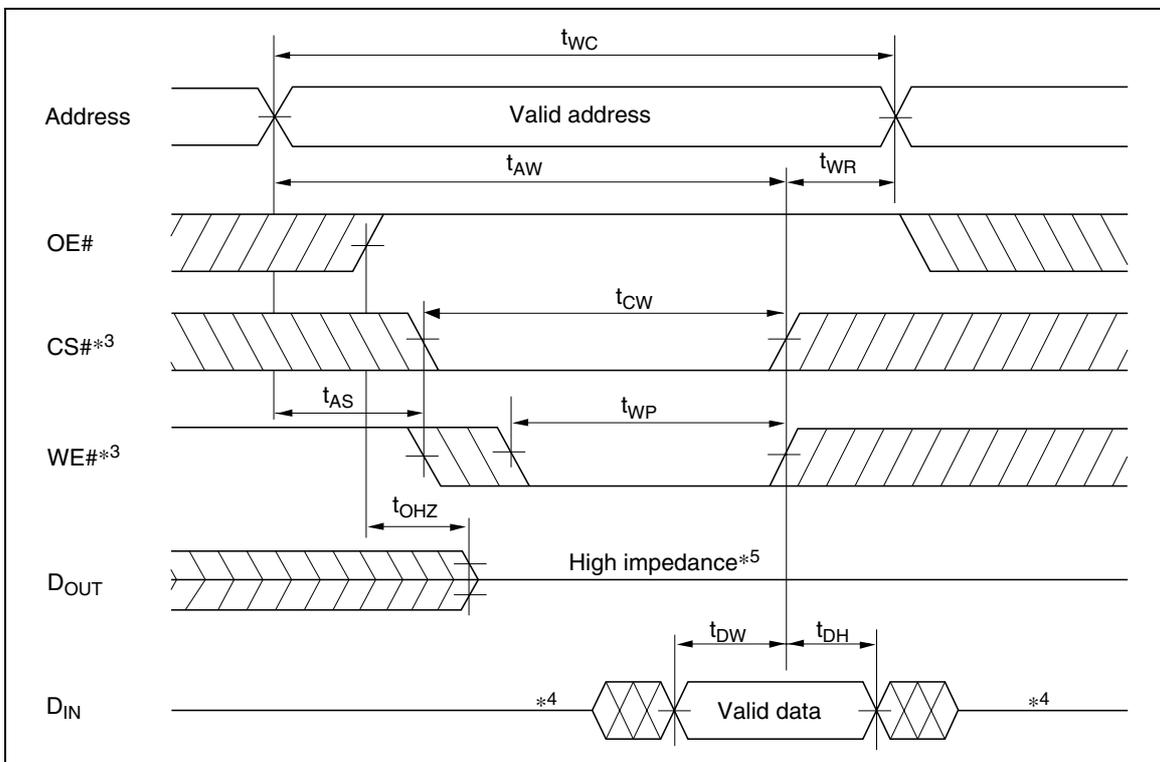
Write Timing Waveform (2) (CS# Controlled)
