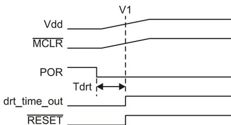
**Figure 13-4: Time-Out Sequence on Power-Up**
