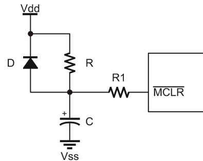
**Figure 13-5: External Power-On Reset Circuit**
