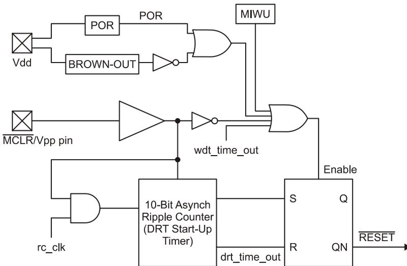
**Figure 13-2 Block Diagram of On-Chip Reset Circuit**
