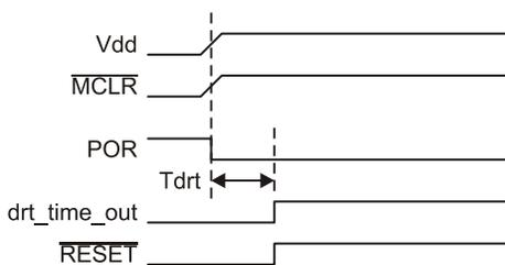
**Figure 13-3: Time-Out Sequence on Power-Up**
