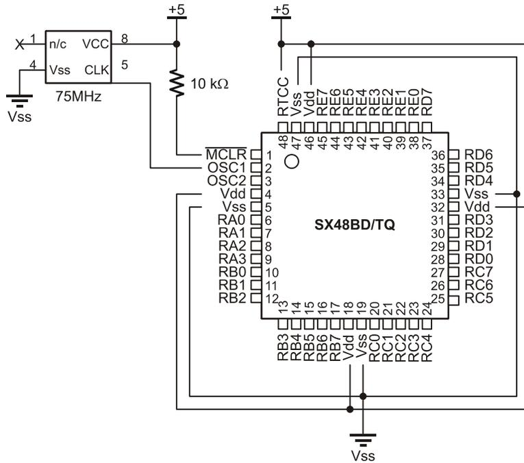
Figure 9-3: SX48BD with 75 MHz TTL Oscillator
