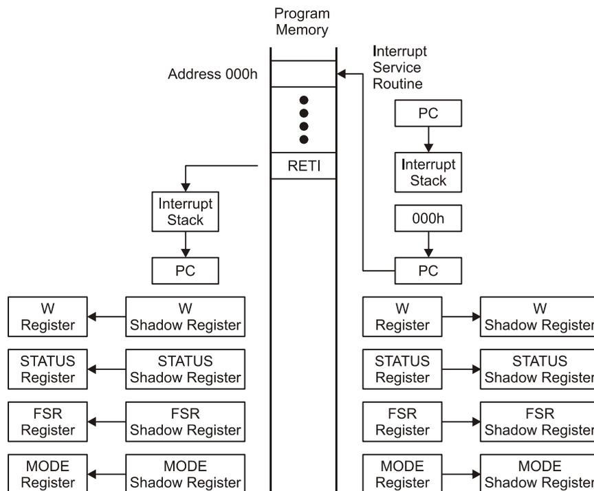
**Figure 8-2: Interrupt Processing**
