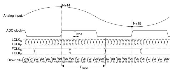
Figure 6. LVDS timing 12 bit output, SDR mode
