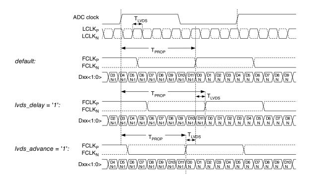
Figure 10. LVDS output timing adjustment
