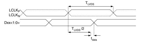
Figure 7. LVDS data timing, DDR mode
