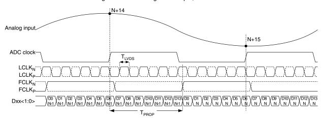
Figure 5. LVDS timing 14 bit output, DDR mode
