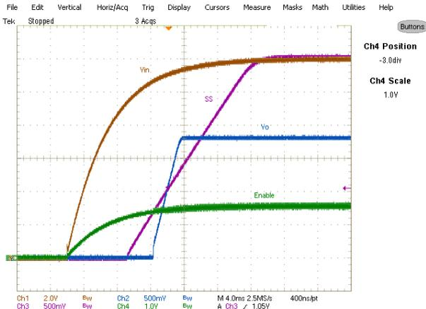
Fig. 18: Start up at 6A Load
