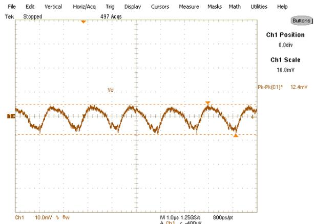
Fig. 21: Output Voltage Ripple, 6A load Ch<sub>1</sub>: V<sub>out</sub>
