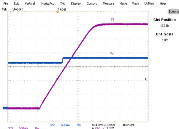
Fig. 20: Start up with 1.62V Pre-Bias, 0A Load, Ch<sub>2</sub>:V<sub>out</sub>, Ch<sub>3</sub>:V<sub>ss</sub>
