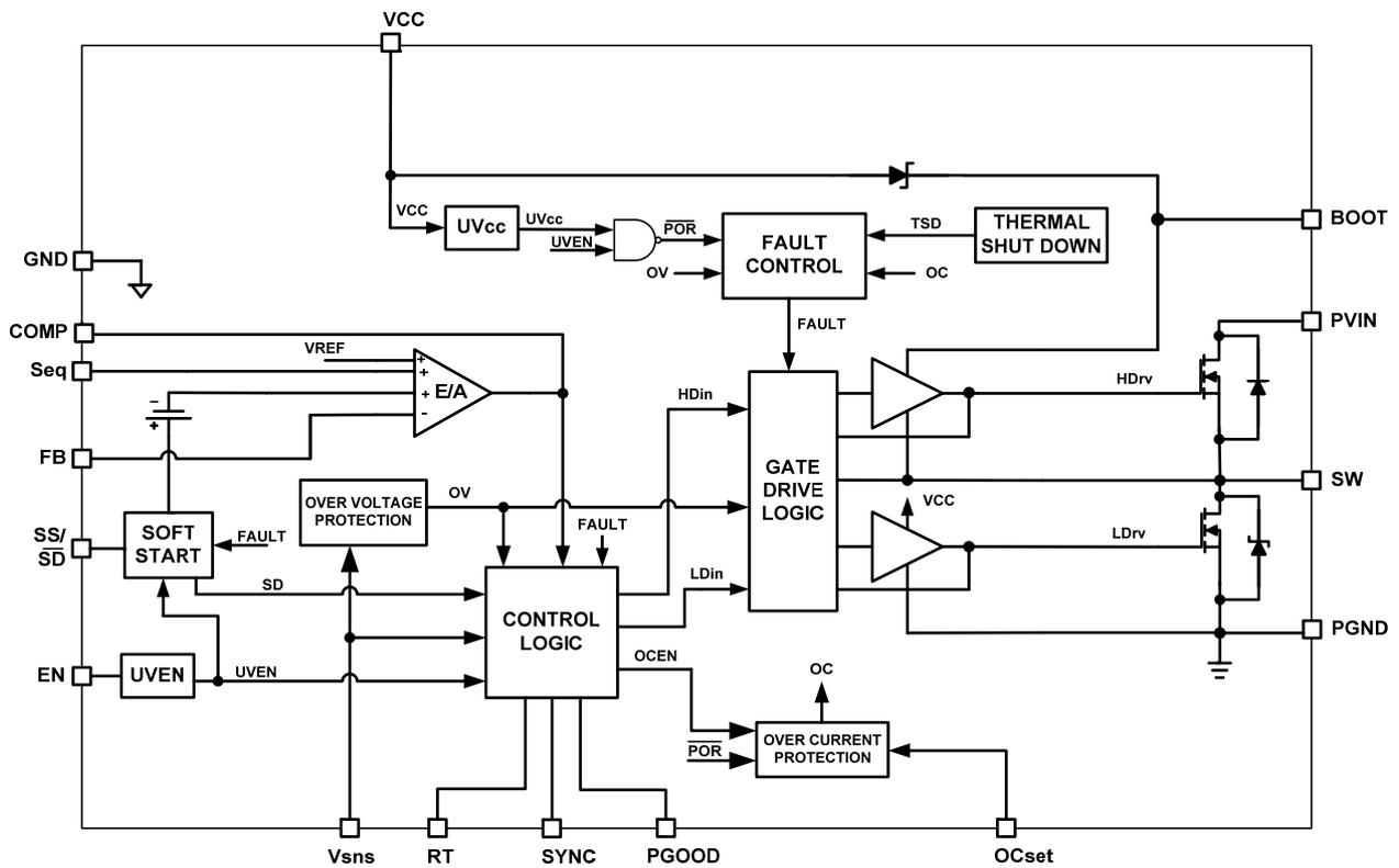
Fig. 2. Simplified block diagram of the IR3856
