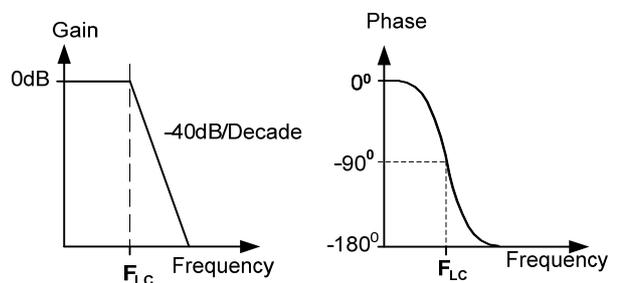
Fig. 14. Gain and Phase of LC filter
