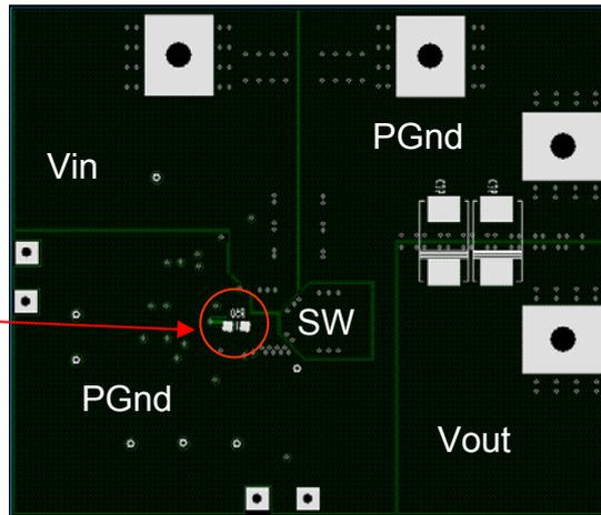
Fig. 28b. IRDC3856 demoboard layout considerations – Bottom Layer
