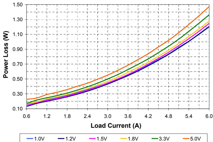
**Typical Efficiency and Power Loss Curves**
