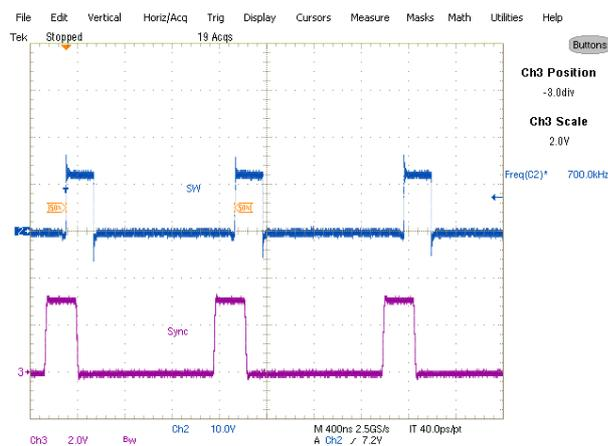
Fig. 26: Synchronization to 700kHz external clock signal at 6A load
