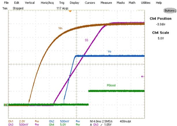
Fig. 19: Start up at 6A Load,
