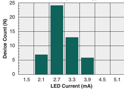
Typical  $I_F$  for Switch Dropout
