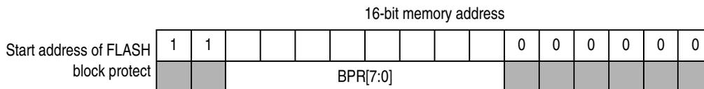
The resultant 16-bit address is used for specifying the start address of the FLASH memory for block protection. The FLASH is protected from this start address to the end of FLASH memory, at \$FFFF. With this mechanism, the protect start address can be XX00, XX40, XX80, or XXC0 (at page boundaries — 64 bytes) within the FLASH memory.
