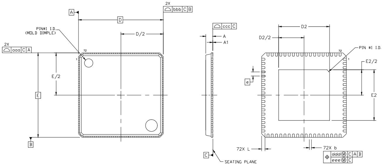
**Figure 12. 72-Pin Quad Flat No Lead (QFN) Package**
