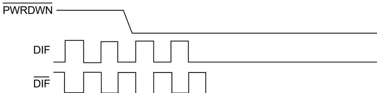
**Figure 1.  $\overline{\text{PWRDN}}$  Assertion**
