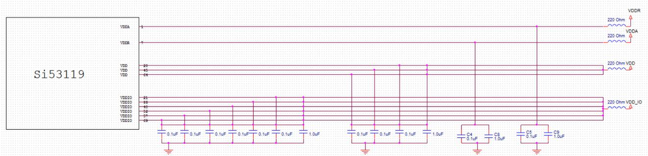
Figure 11. Schematic Example of the Si53119-A03A Power Filtering
