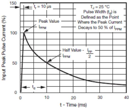
Fig. 3 - Pulse Waveform
