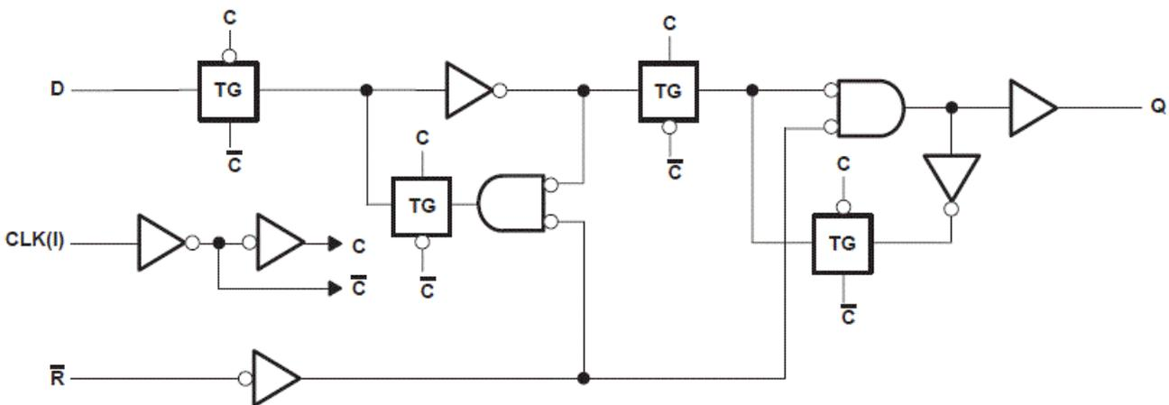
Figure 8-2. Logic Diagram, each flip-flop (positive logic)
