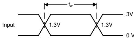
**Figure 7-2. Voltage Waveforms, TTL-Compatible CMOS Inputs Pulse Duration**
