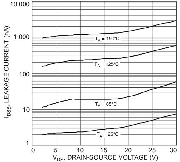
Fig. 8 Typical Drain-Source Leakage Current vs Voltage
