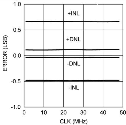
**Figure 8. INL/DNL vs  $f_{SCLK}$  at  $V_A = 2.7\text{ V}$**
