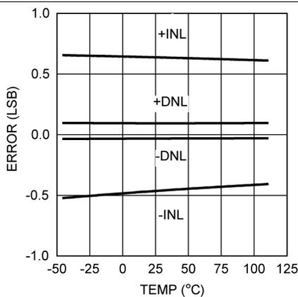
**Figure 12. INL/DNL vs Temperature at  $V_A = 3\text{ V}$**
