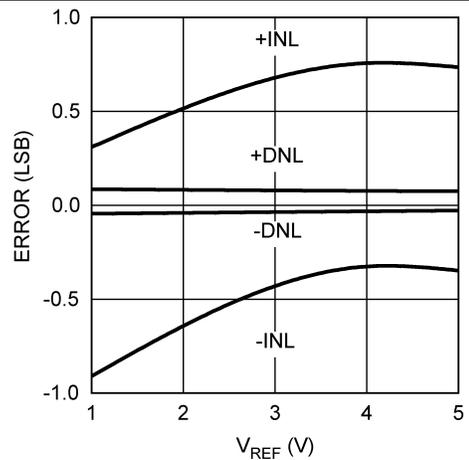
Figure 7. INL/DNL vs  $V_{REFIN}$  at  $V_A = 5$  V
