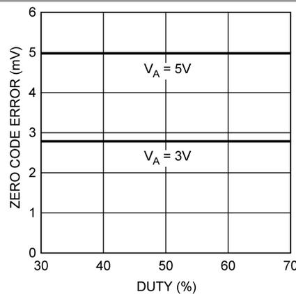
Figure 17. Zero Code Error vs Clock Duty Cycle
