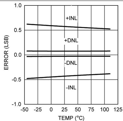
**Figure 13. INL/DNL vs Temperature at  $V_A = 5\text{ V}$**
