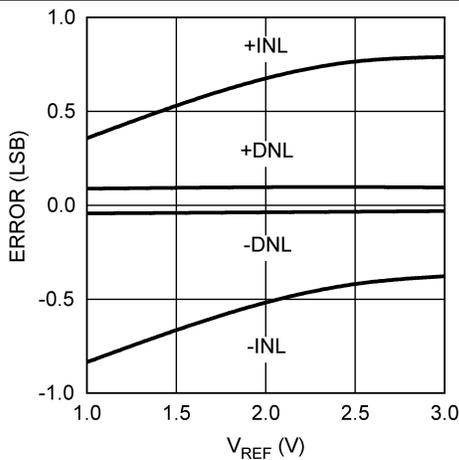
Figure 6. INL/DNL vs  $V_{REFIN}$  at  $V_A = 3$  V
