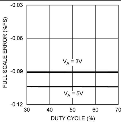
Figure 22. Full-Scale Error vs Clock Duty Cycle
