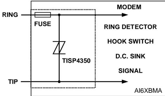
Figure 14. Modem Inter-wire Protection
