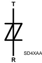
Terminals T and R correspond to the alternative line designators of A and B
