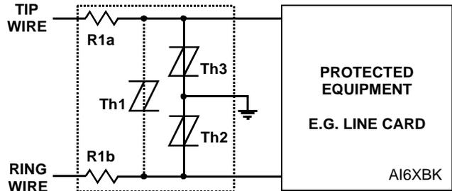
Figure 15. Protection Module
