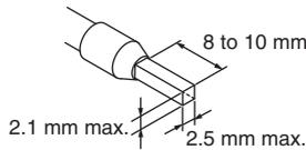
3. For the ferrule which is for applicable wire (1 to 1.5 mm<sup>2</sup>/ AWG 18 to 16), please use a ferrule without an insulation sleeve. (Refer to the following table.)
