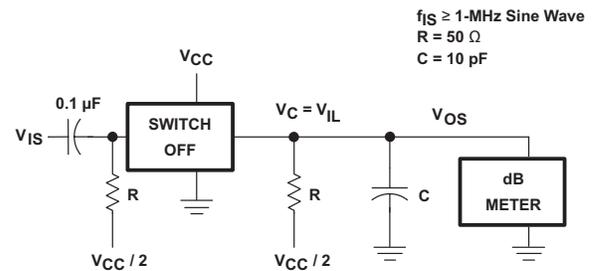
Figure 4. Switch OFF Signal Feedthrough Test Circuit
