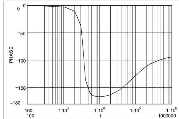
**FIGURE 4-6:** Phase Curve with ESR =  $0.002\Omega$ .
