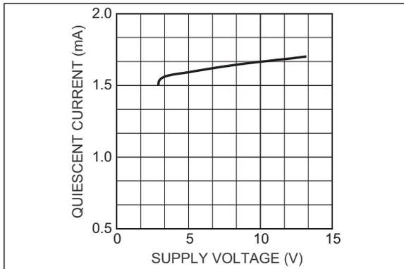
**FIGURE 2-2:** PWM Mode Supply Current vs. Supply Voltage.
