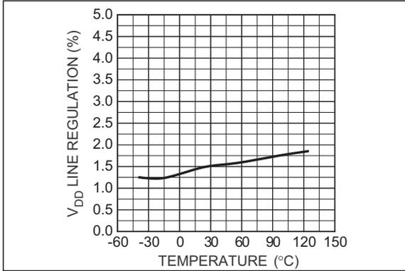
**FIGURE 2-7:** *V<sub>DD</sub> Line Regulation vs. Temperature.*
