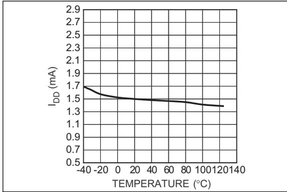
**FIGURE 2-1:** PWM Mode Supply Current vs. Temperature.
