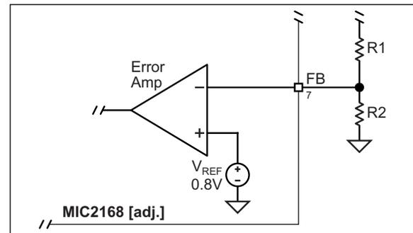
**FIGURE 4-2:** Voltage-Divider Configuration.
