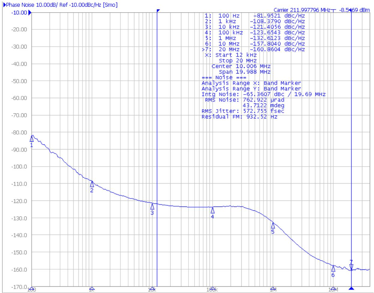
Figure 3. Typical Phase Noise Plot at 212.00 MHz
