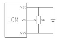
VDD~V0: LCD Driving voltage
