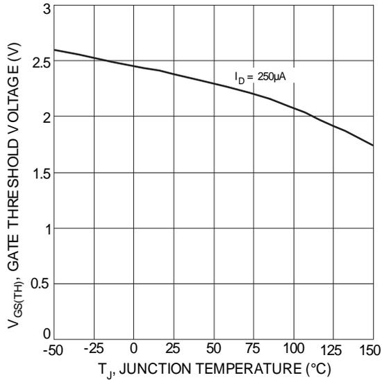
Figure 7 Gate Threshold Variation vs. Ambient Temperature
