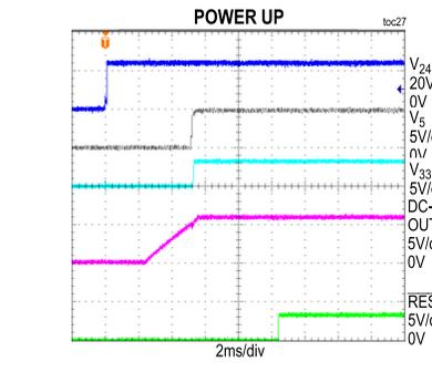
$V_{24} = 24V$ , DC-DC regulator is enabled and connected to LIN,  $V_L = V_{33}$ ,  $T_A = +25^\circ C$ , unless otherwise noted.
