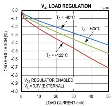
$V_{24} = 24V$ , DC-DC regulator is enabled and connected to LIN,  $V_L = V_{33}$ ,  $T_A = +25^\circ C$ , unless otherwise noted.
