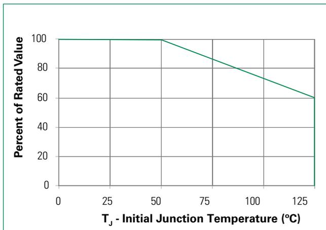
**Figure 4 - Typical Peak Pulse Power Rating Curve**
