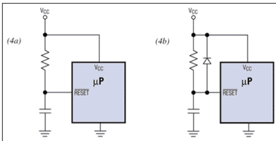
Figure 4. The discrete R/C POR (Figure 4a) is not reliable enough for most applications. In some cases,
