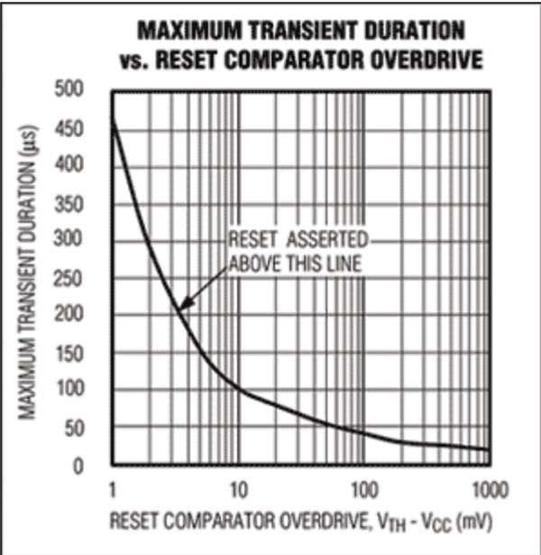
Figure 2. Whether a POR generates a reset is a function of both the amplitude and duration of the glitch.
