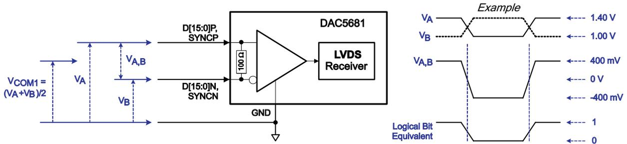
Figure 27. LVDS Data (D[15:0]P/N, SYNCN/P Pairs) Input Levels
