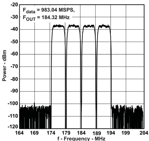
Figure 14. Four Carrier W-CDMA Test Model 1
