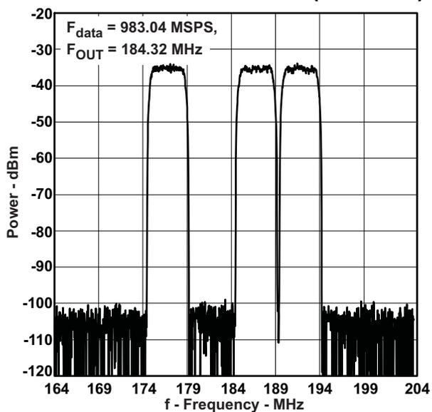
Figure 15. Three Carrier W-CDMA Test Model 1 with GAP
