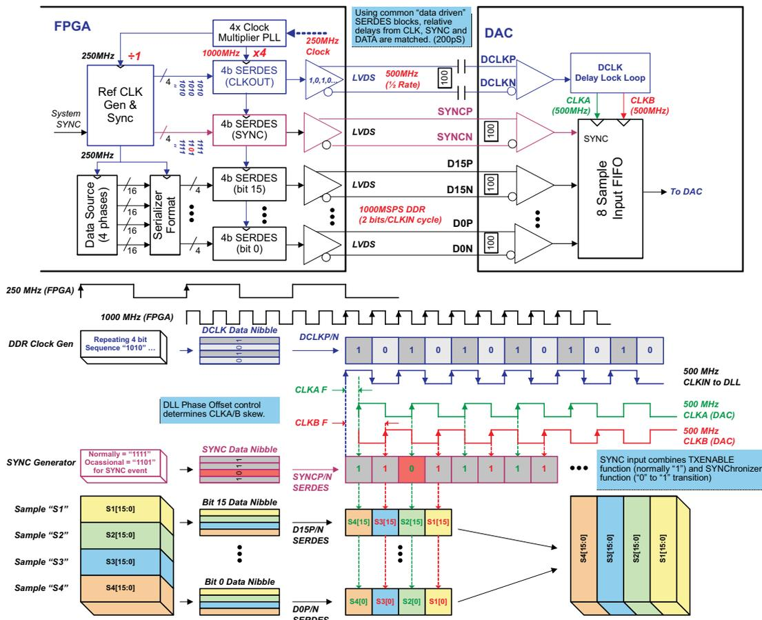
Figure 25. Example FPGA-Based LVDS Data Flow to DAC
