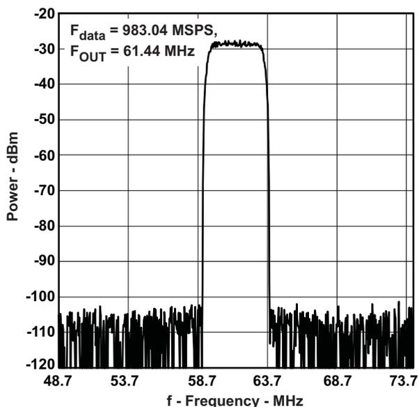
Figure 11. Single Carrier W-CDMA Test Model 1
