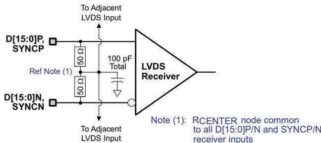
Figure 26. D[15:0]P/N and SYNCP/N LVDS Input Configuration
