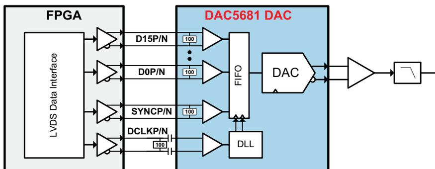
Figure 35. System Diagram of Arbitrary Waveform Generator
