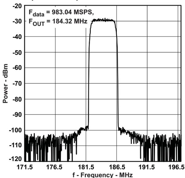
Figure 12. Single Carrier W-CDMA Test Model 1
