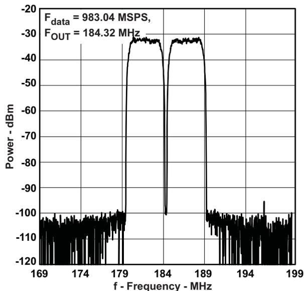
Figure 13. Two Carrier W-CDMA Test Model 1
