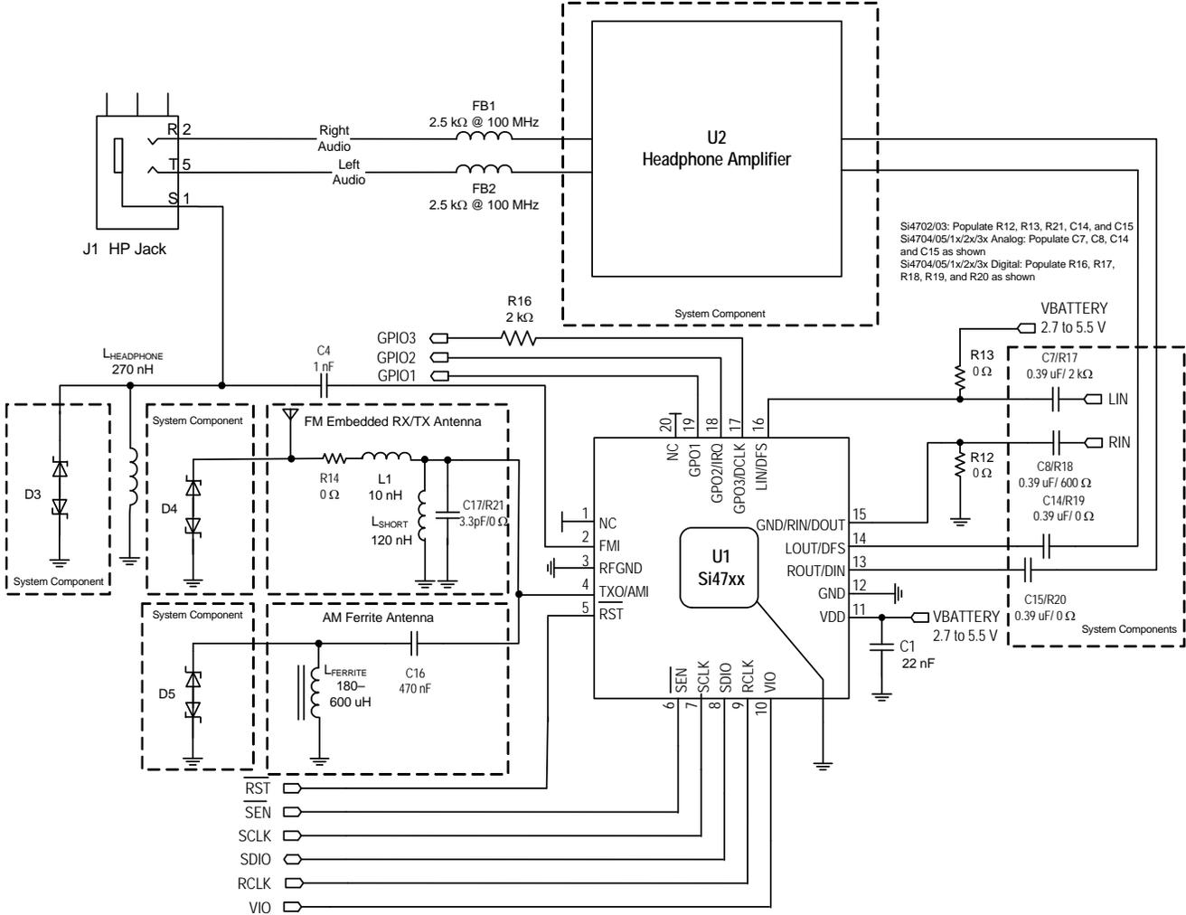
Figure 12. Universal AM/FM RX/FM TX Application Schematic
