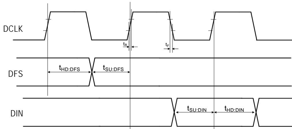
**Figure 8. Digital Audio Interface Timing Parameters, I<sup>2</sup>S Mode**
