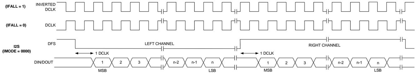
**Figure 14. I<sup>2</sup>S Digital Audio Format**
