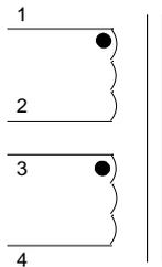
\*For 0.024H at 20Amp, connect to 1 to 4, Jumper 2 to 3
