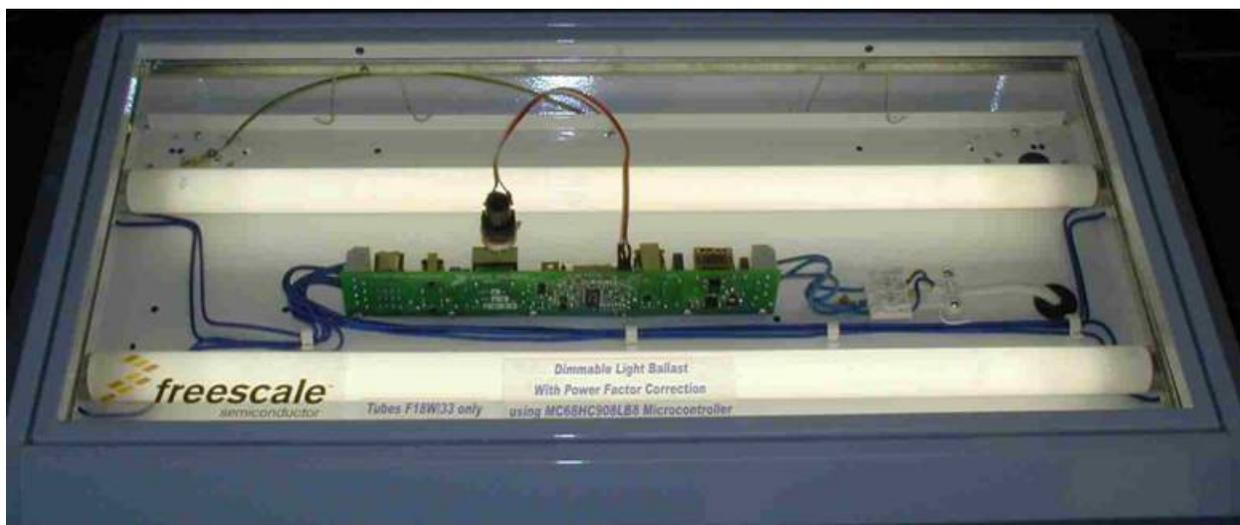
**Figure 1-1. Dimmable Light Ballast with PFC Demo**
