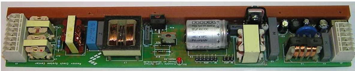
**Figure 4-1. Dimmable Light Ballast - Demo Board**
