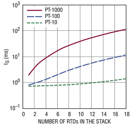
Figure 3. Simulated Settling Time of the RTD Stack
